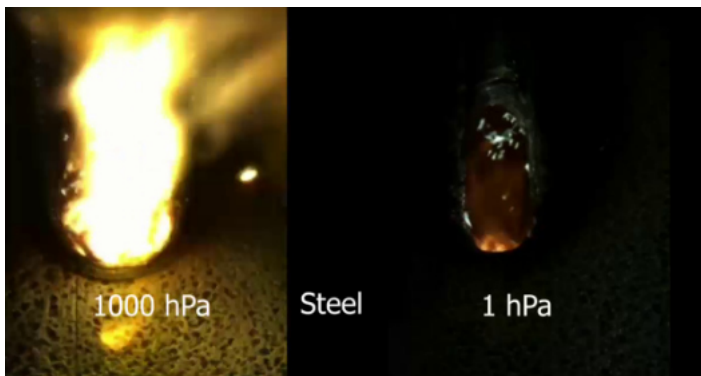
The laser welding process for steel & copper performed at atmospheric pressure (1000 hPa) compared to vacuum conditions (1 hPa).
