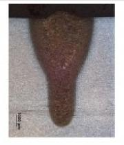
Gallery: A drop in pressure changes the shape of the seam cross section.
