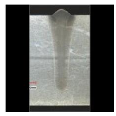
Gallery: Penetration welding in the pressure range from 1030 to 10 millibar
